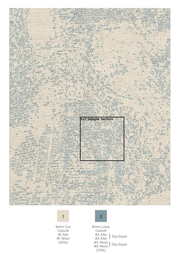
This technical drawing represents color placement and fiber construction including the multiple plies used to create the intricate tweed and strie shown in samples.
