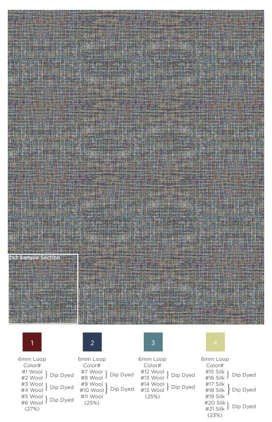
This technical drawing represents color placement and fiber construction including the multiple plies used to create the intricate tweed and strie shown in samples.
