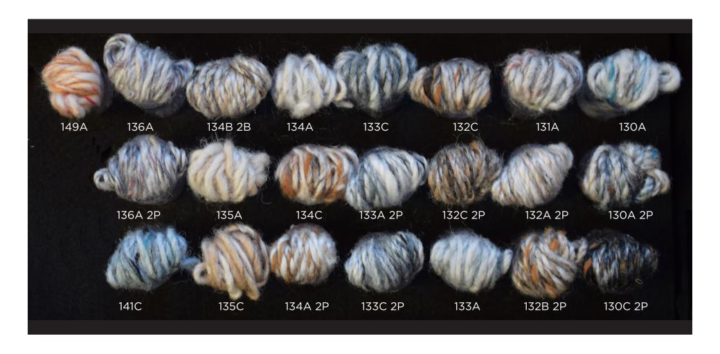
For Indoor & Outdoor use providing excellent performance PET Yarn (Polyethylene Terephthalate) is a material that is made from recycled plastic bottles. Characteristics include: Superb strength, colorfastness and soft texture. It is non-allergenic. A tolerance for water or moisture and resistance to staining, fading, mold, mildew, abrasion and sunlight. It is sustainable and recyclable.
